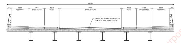
Figure 10: Composite Steel Girder and In-situ Deck
