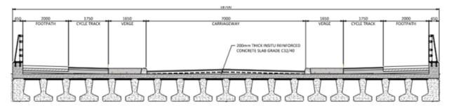
Figure 9: Precast Beams and In-situ Deck
